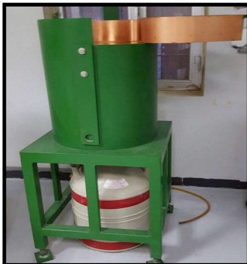
Figure 3. The HPG detector shielded with lead to prevent the background radiation from reaching the samples.
