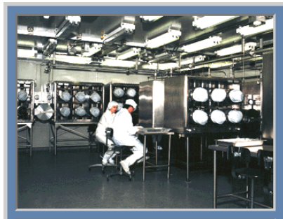
Figure 2. Lunar sample storage and processing system in the US Lunar Sample Laboratory
