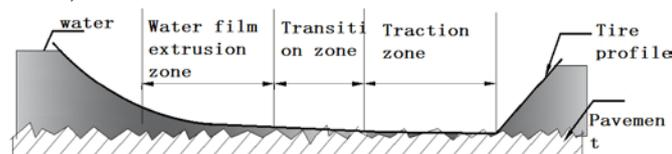
Fig 1. Schematic diagram of the three zones where the tire is in contact with the watery road
