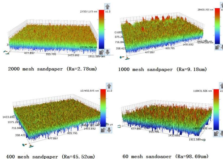
**Fig 2.** Three-dimensional surface topography of the samples after pre-grinding
