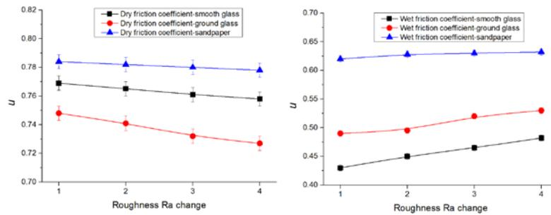
**Fig 4.** Variation curve of friction coefficient with sample surface roughness
