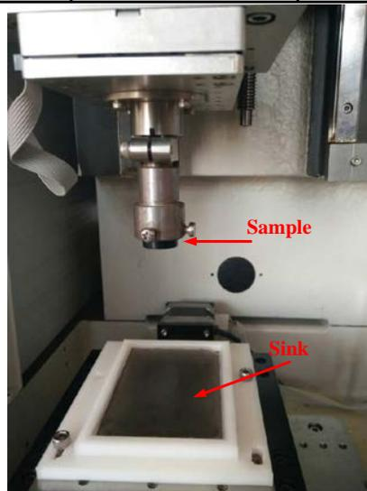
**Fig 3.** The wet and dry sliding friction test device
