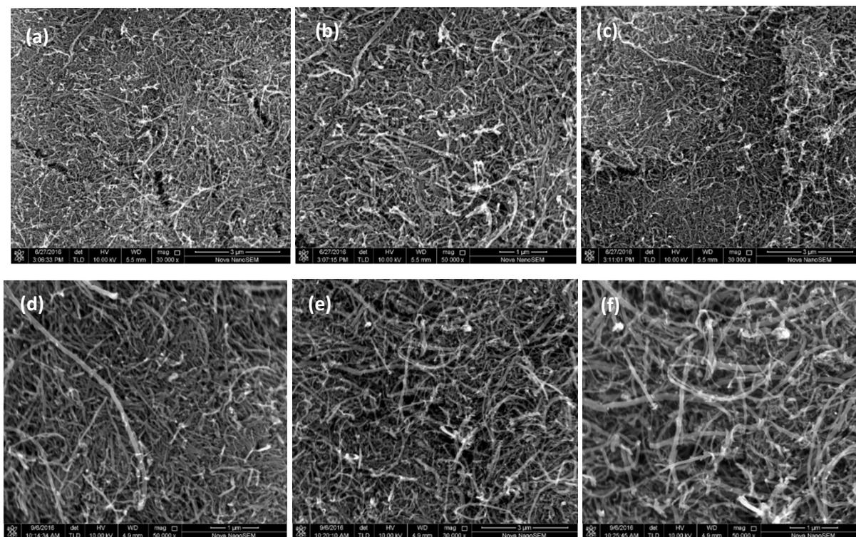
Figure 1 Microscopic morphology of CNTs after chemical functionalization
