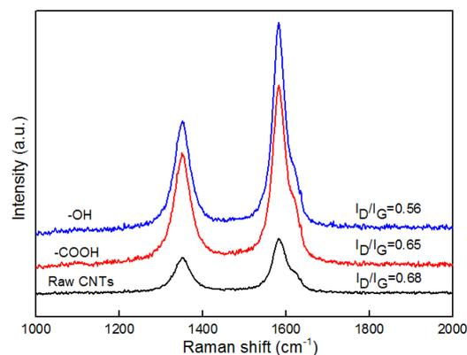
Figure 3 Raman spectra of CNTs after chemical functionalization
