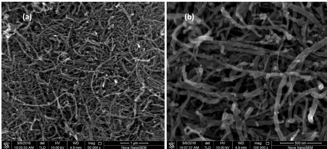
Figure 4 Microscopic morphology of CNTs after high-temperature graphitization treatment
