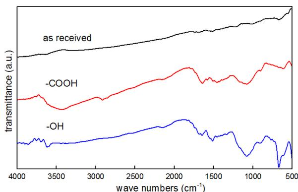
Figure 2 Infrared spectrum of CNTs after chemical functionalization
