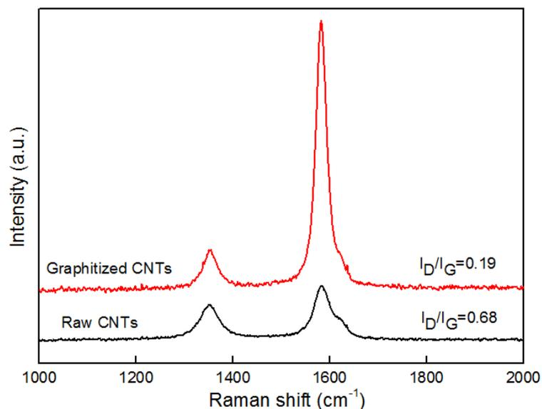
Figure 5 Raman spectrum of the original state and the graphitized CNTs.
