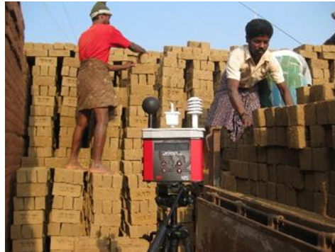
Figure 2. WBGT measurement instrument (QUESTemp) at one of the brick kilns studied.
