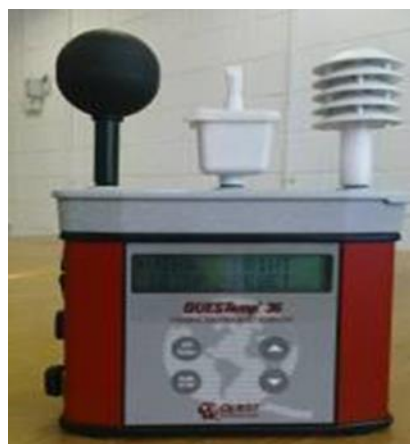
Figure 9. Quest-Thermal Environment monitor (Heat stress monitor).
