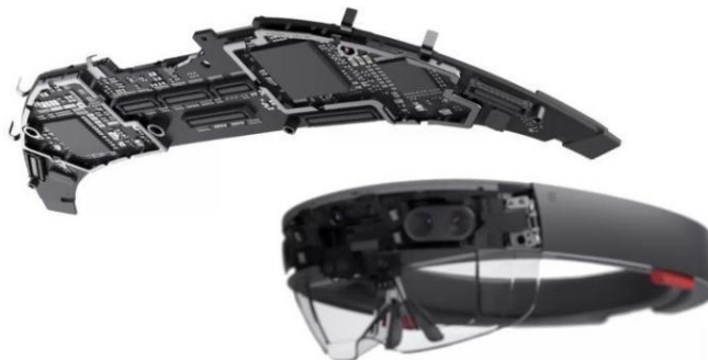
Figure 1. HoloLens holographic processing unit
