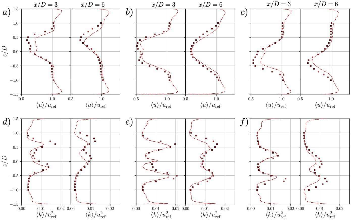
**Figure 5.** Horizontal profiles of the time-averaged streamwise velocity (a-c) and the turbulent kinetic energy (d-f) at  $3D$  and  $6D$  behind the turbine under inflow (iii) for the three yaw angles configuration: a,d)  $\gamma = -30^\circ$ , b,e)  $\gamma = 0^\circ$  and c,f)  $\gamma = +30^\circ$ . Experimental ( $\blacksquare$ ) and LES ( $-\cdot-\cdot-$ ) results are presented.
