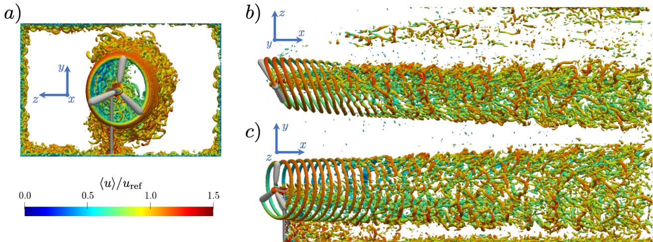
**Figure 3.** Front a), upper b) and side c) views of the instantaneous 3D visualization of the wake generated by the turbine blades, tower and nacelle at  $\gamma = -30^\circ$  under inflow (i) using an iso-contour of the  $Q$  criterion colored by flow velocity. The grey iso-surface represents a contour of the volume force applied to the flow by the blades. The tower and nacelle surfaces are in dark grey.
