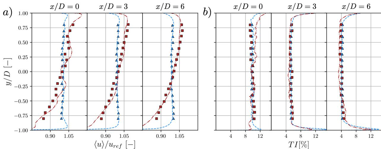
**Figure 2.** Vertical profiles of the time-averaged a) streamwise velocity and b) the streamwise turbulent intensity in the wind tunnel without the turbine. The results of the inflows generated with the turbulence grids are presented: (ii) Experimental ( $\blacktriangle$ ), LES (---); (iii) Experimental ( $\blacksquare$ ), LES (-.-.)
