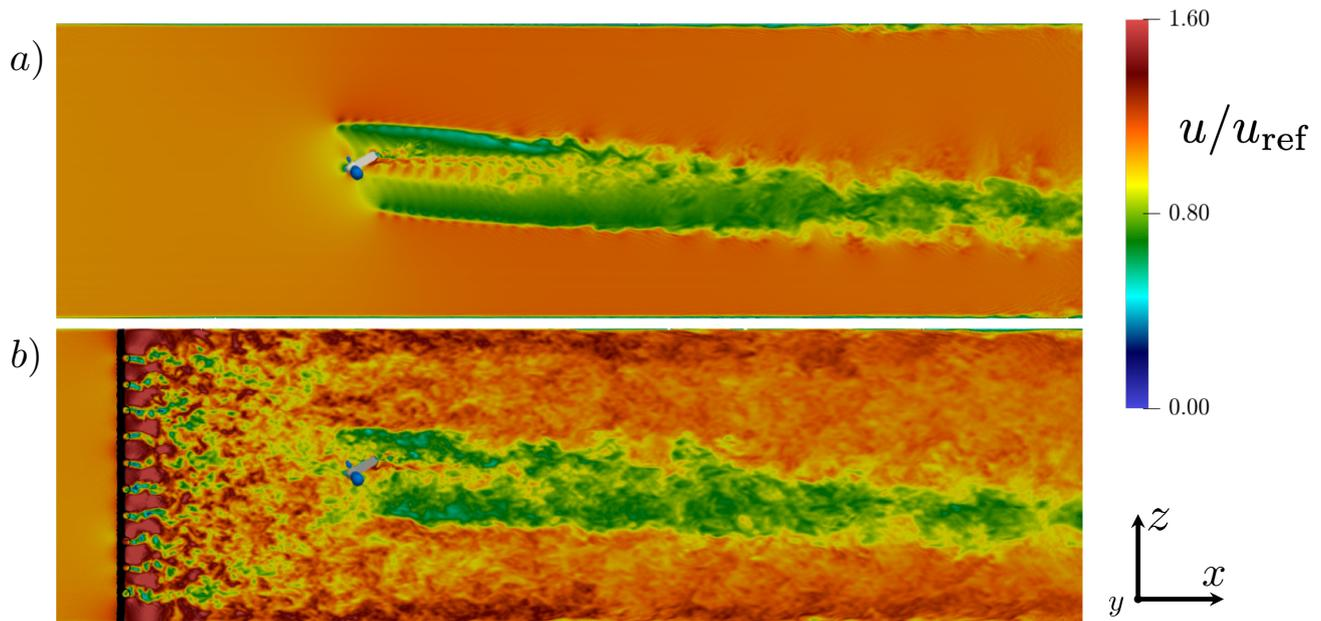
**Figure 4.** Horizontal slice of the instantaneous velocity at  $\gamma = -30^\circ$  under inflows: a) (i) and b) iii). The blue and black iso-surfaces of the flow volume force represent the blade and the turbulence grid, respectively. The tower and nacelle meshed surfaces appear in grey.
