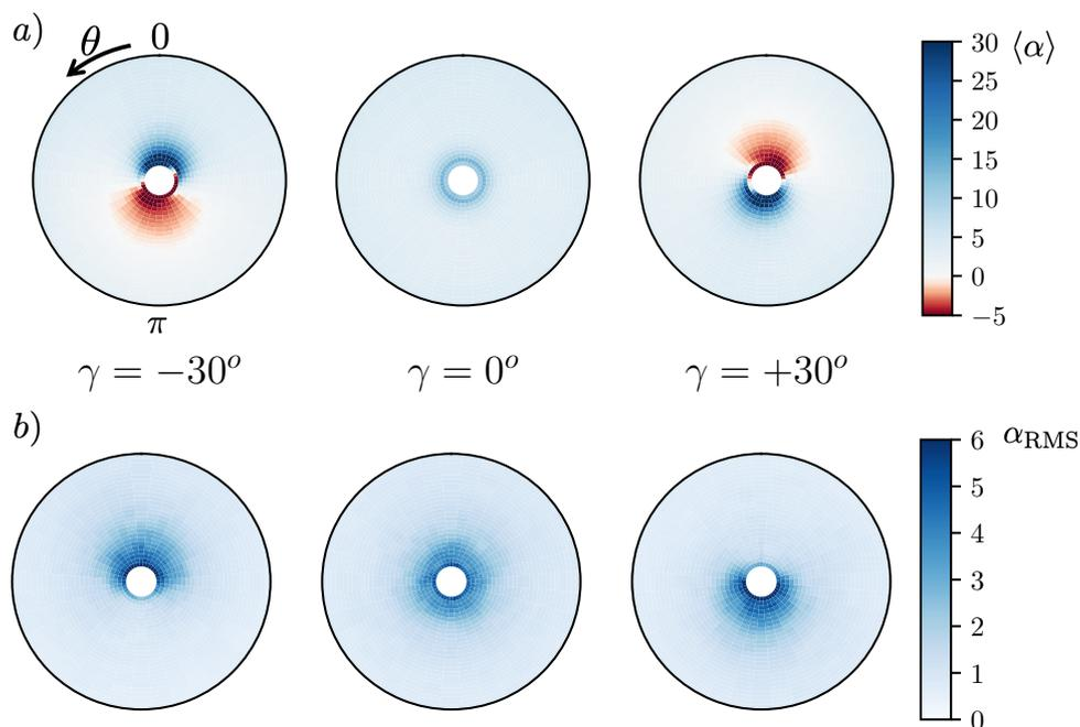
**Figure 7.** Radius and azimuth averaged temporal mean (a) and temporal RMS (b) of angle of attack for  $\gamma = 30^\circ$ ,  $0^\circ$  and  $-30^\circ$  under a non-uniform sheared inflow with a high turbulence level, inflow iii).
