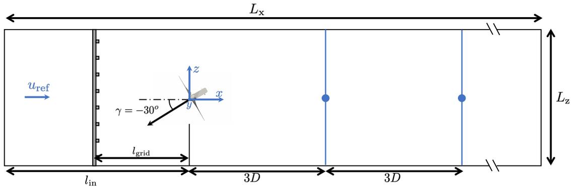
**Figure 1.** Top view of yawed turbine setup according to the reference coordinate system in the wind tunnel. Blue lines (horizontal profiles) and dot (vertical profiles) at  $3D$  and  $6D$  indicate where the time-averaged streamwise velocity and streamwise turbulent stress are extracted. The position of the turbulence grids for inflow (ii) and (iii) are represented. The wind tunnel dimensions are  $L_x \times L_y \times L_z = 14 \times 1.801 \times 2.71 \text{ m}^3$ .
