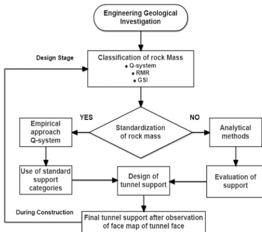
**Figure 3.** Design Process for estimation of tunnel support [4].
