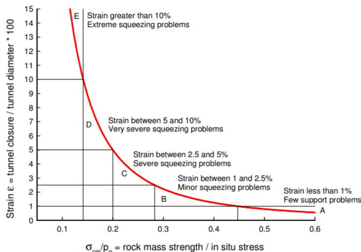
**Figure 2.** Semi-empirical method for classifying rocks based on strain values [16].
