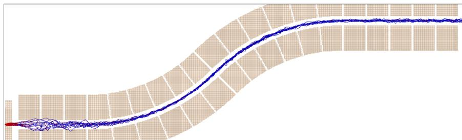
**Figure 5.** S-shaped RFQ and ion trajectories within it. Radiofrequency (0.67 MHz) voltage amplitude is set to 300 V, with overall longitudinal gradient of 20 V. Buffer gas (argon) pressure inside the gas cell is 500 mbar, and the pressure in the vacuum chamber is  $10^{-2}$  mbar.
