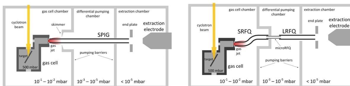
**Figure 4.** Two designs of the ion guide: SPIG (on the left-hand side) and S-shaped RFQ (right-hand side).
