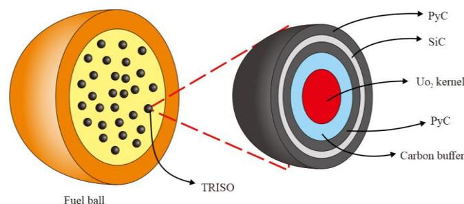
**Figure 1.** HTR-10 fuel element and TRISO particle
