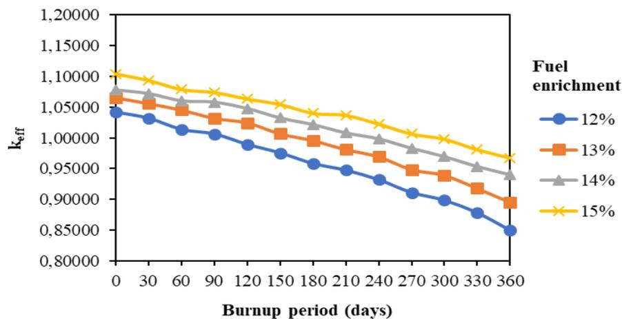
**Figure 6.**  $k_{\text{eff}}$  value as the function of fuel enrichment in a 250  $\mu\text{m}$  kernel radius.
