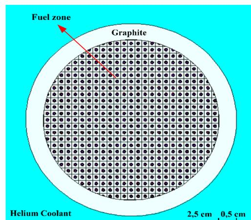
**Figure 3.** Representation of the fuel ball model used in MCNP.
