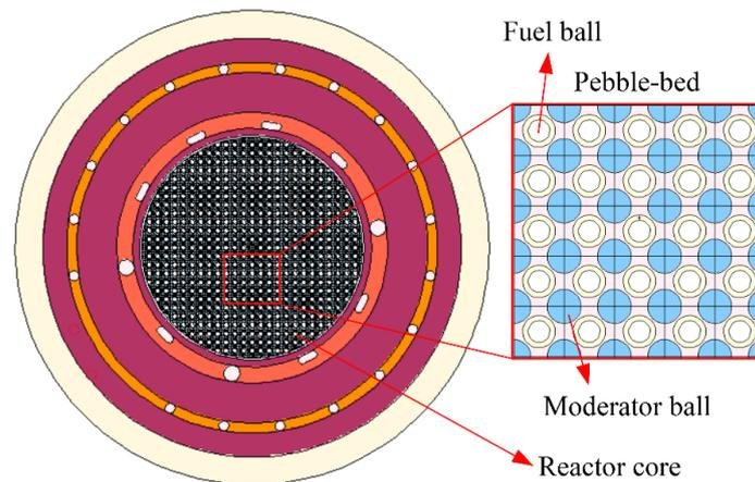
**Figure 4.** Representation of the horizontal cross-section of the HTR-10 model used in MCNP.
