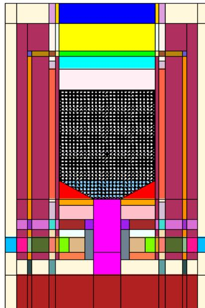
**Figure 5.** Representation of the vertical cross-section of the HTR-10 model used in MCNP.
