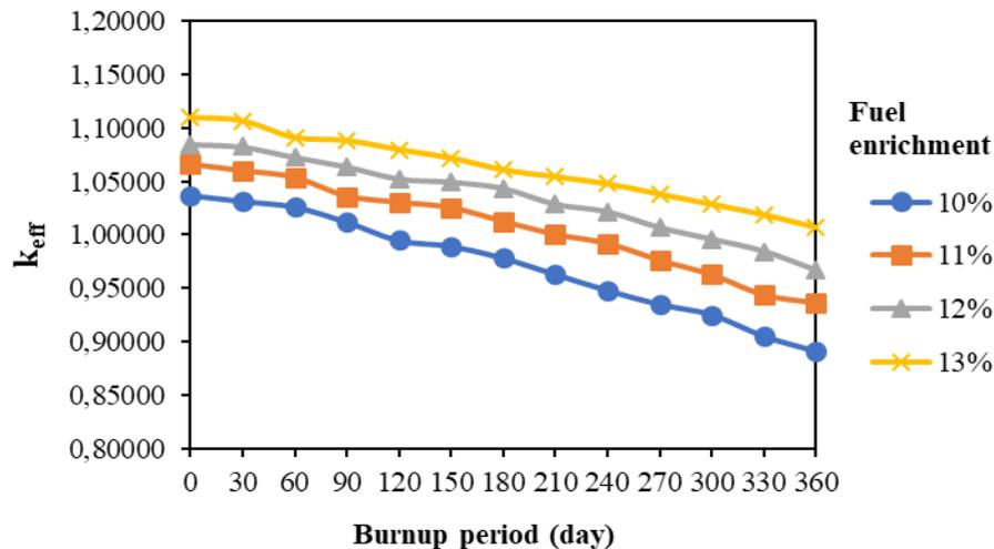
**Figure 8.**  $k_{\text{eff}}$  value as the function of fuel enrichment in a 300  $\mu\text{m}$  kernel radius.
