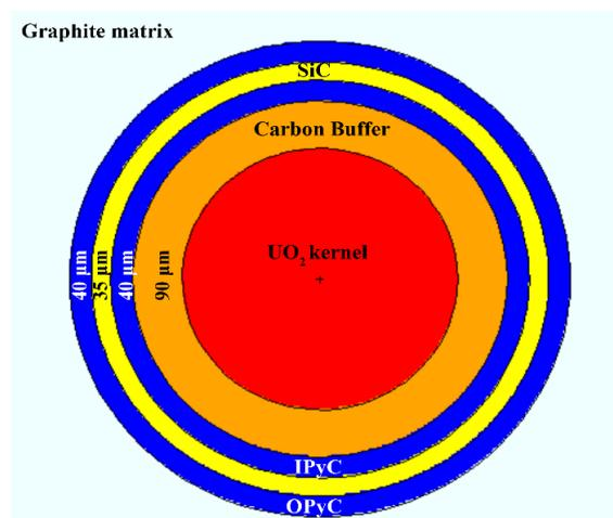
**Figure 2.** Representation of the TRISO particle model used in MCNP.
