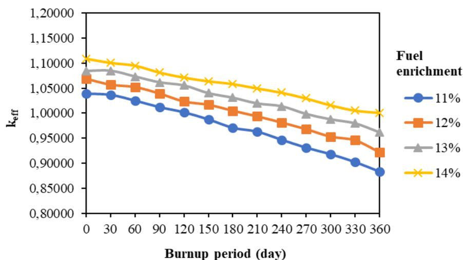
**Figure 7.**  $k_{\text{eff}}$  value as the function of fuel enrichment in a 275  $\mu\text{m}$  kernel radius.
