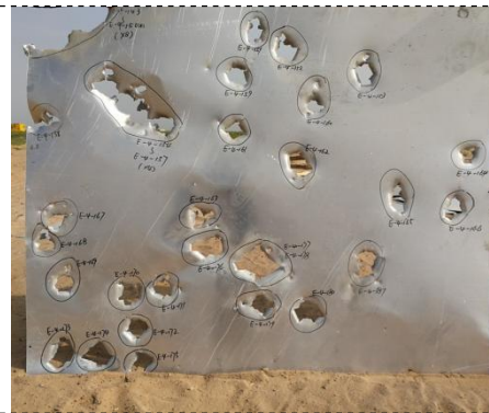
Figure 13. Typical Damage effect on Aluminum sheet.
