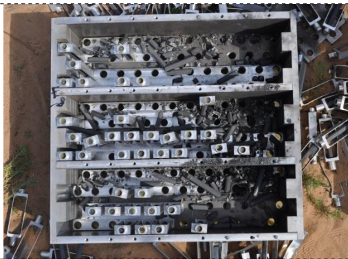
Figure 12. Damage effect on phased array radar antenna module.
