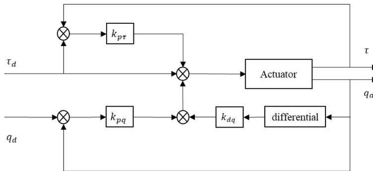
Figure 2. the principle block diagram of the force-bit hybrid control.
