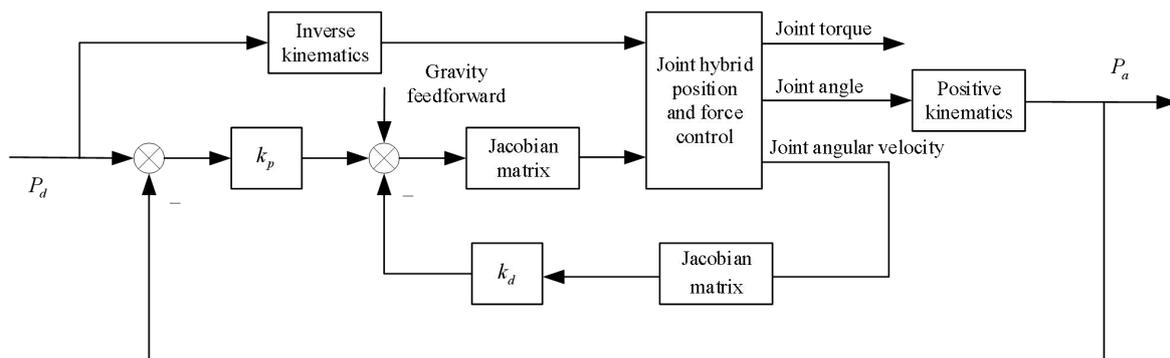
Figure 3. Impedance Control Based on Foot Position Planning.
