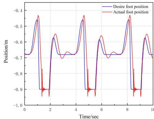
**Figure 7.** Foot position curve with continuous bounce of one leg.
