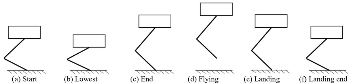
Figure 1. State of each stage of the jumping.
