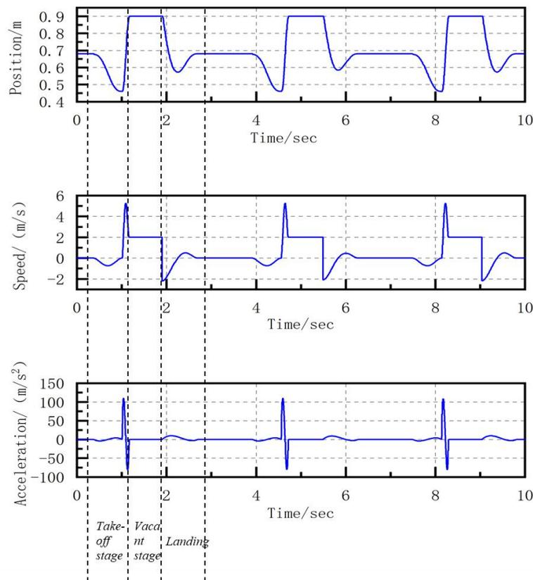
**Figure 6.** Centroid position, velocity, and acceleration with continuous bounce of one leg.
