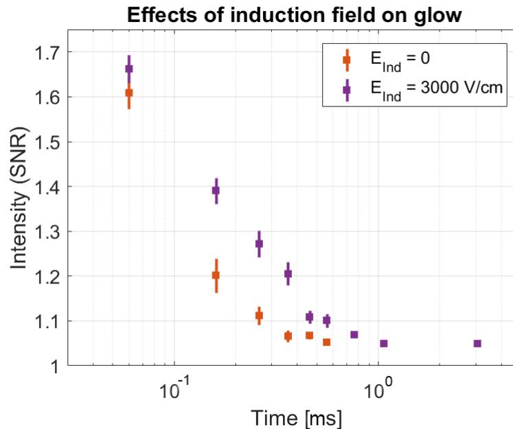
**Figure 7.** The observed glow evolution for Ar-CO<sub>2</sub> (90-10) using Retiga CCD camera. The measurements are conducted with 0 and 3000 V/cm applied induction fields, with the latter being close to the required field strength to produce propagations.
