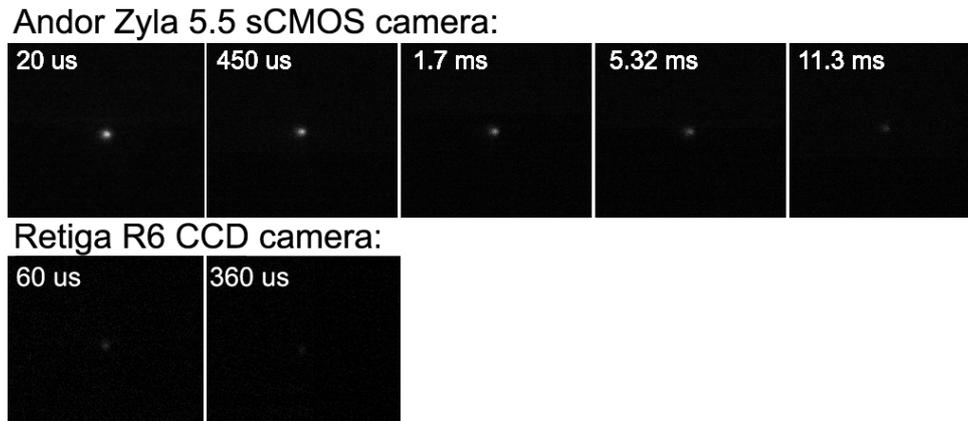
**Figure 6.** The observed time evolution of the glow after a primary discharge compared between two use scientific cameras. Given time information is for the initial signal peak from the primary discharge being in time 0.
