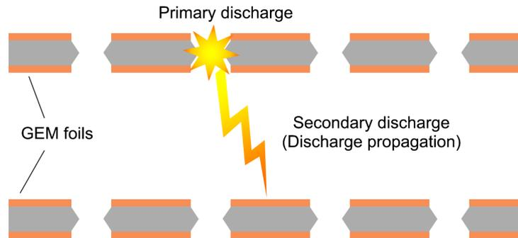
**Figure 1.** Schematic of the two types of GEM discharges.
