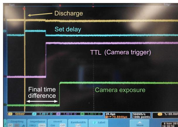
**Figure 5.** The signals used for the triggering of the camera. Yellow: The electrical signal induced by the primary discharge measured at the anode. Blue: Adjustable delay to control the time difference between camera exposure and discharge. Purple: The trigger sent to the camera. Green: Gate from the camera showing the exposure of the sensor.
