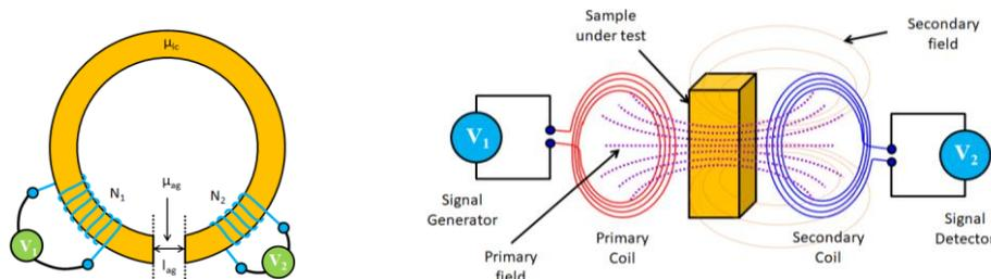
**Fig. 1.** (a) MIS systems for (a) permeability measurement [30], (b) conductivity measurement [31].
