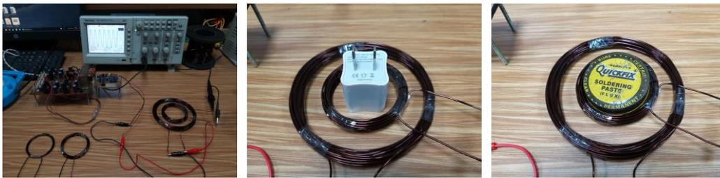
Fig. 3: (a) MIS experimental set up with 20:20 coil assembly, (b) object 1, (c) object 2.
