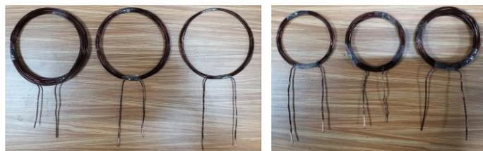
**Fig. 2.** MIS Copper coils (a) primary coils ( $D_{1i} = 94$  mm), (b) secondary coils ( $D_{2i} = 54$  mm).
