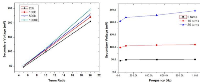
**Fig. 4:** (a) Secondary voltage for different turn ratios in the secondary with a primary coil with 20 turns, (b) Secondary voltage for different frequencies with a turn ratios of 5, 10 and 20.
