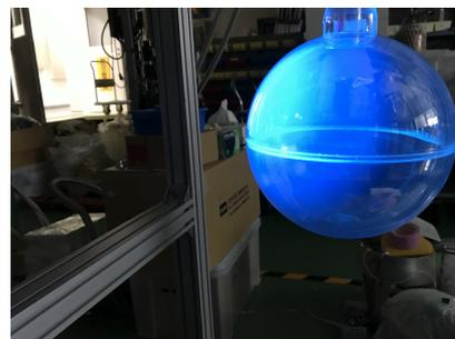
**Figure 3.** Tritan<sup>TM</sup> based plastic scintillator vessel.
