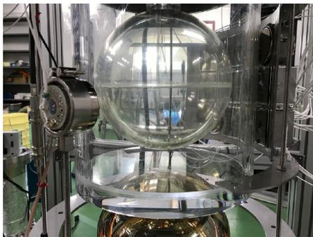
**Figure 4.** Cryostat for Cherenkov light detection. The  $\phi$  20 cm plastic scintillator vessel and transparent adiabatic vacuum vessel.
