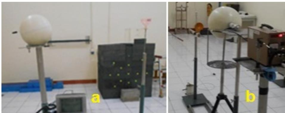
**Figure 4.** Measurement of  $^{252}\text{Cf}$  neutron spectra using SSS (a) and BSS (b).
