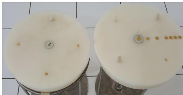
**Figure 1.** A prototype of SSS with 7 Au foils
