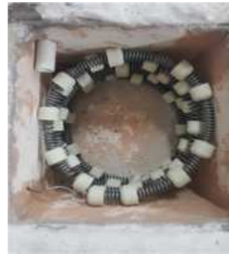
Figure 1. b. The inner of the furnace, which is 9 cm high and 12 cm wide
