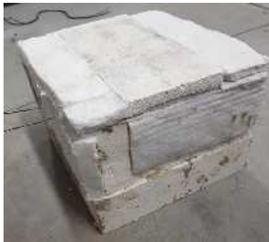
Figure 1. a. Glass melting furnace, which is 14 cm high and 23 cm wide
