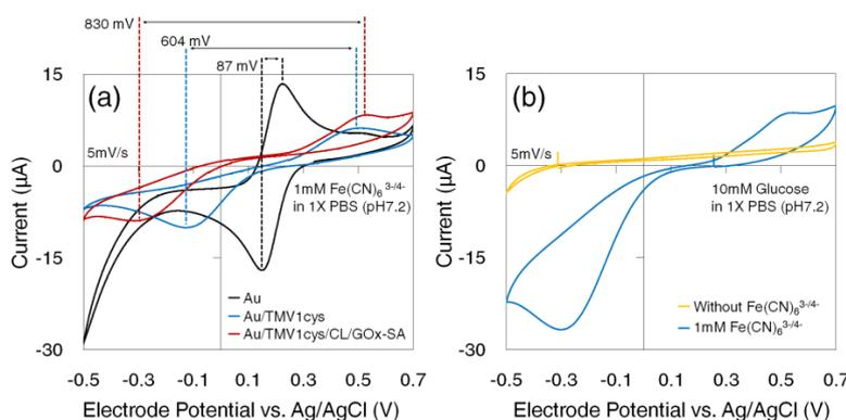
**Figure 3.** Electrochemical characterization showing (a) a change in charge transfer kinetics with electrode functionalization and (b) effective charge transfer mechanism for the Au/TMV1cys/CL/GOx-SA electrodes.
