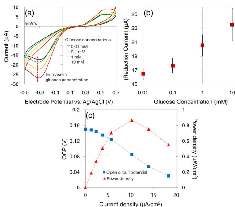
**Figure 4.** Electrochemical characterizations showing (a, b) increase in redox currents corresponding to glucose concentrations and (c) a polarization curve acquired from Au/TMV1cys/CL/GOx-SA (anode) – Pt (cathode) assembled EBC.
