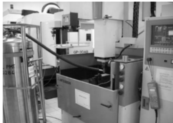
Figure 2: Experimental Set-up showing the application Cryogenic Cooling in Machining [7].
