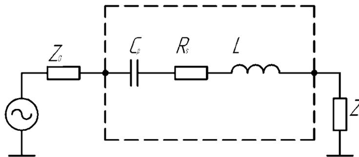
**Figure 2.** Equivalent Capacity Scheme.
