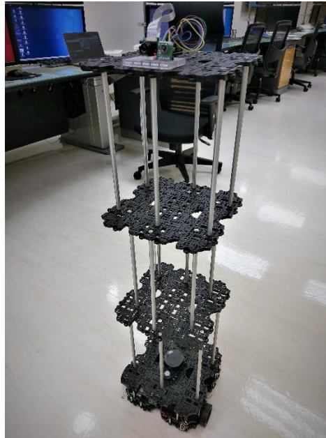
Figure 6. PhotonBot after adding three vertical extensions to increase its height to 1100 mm.
