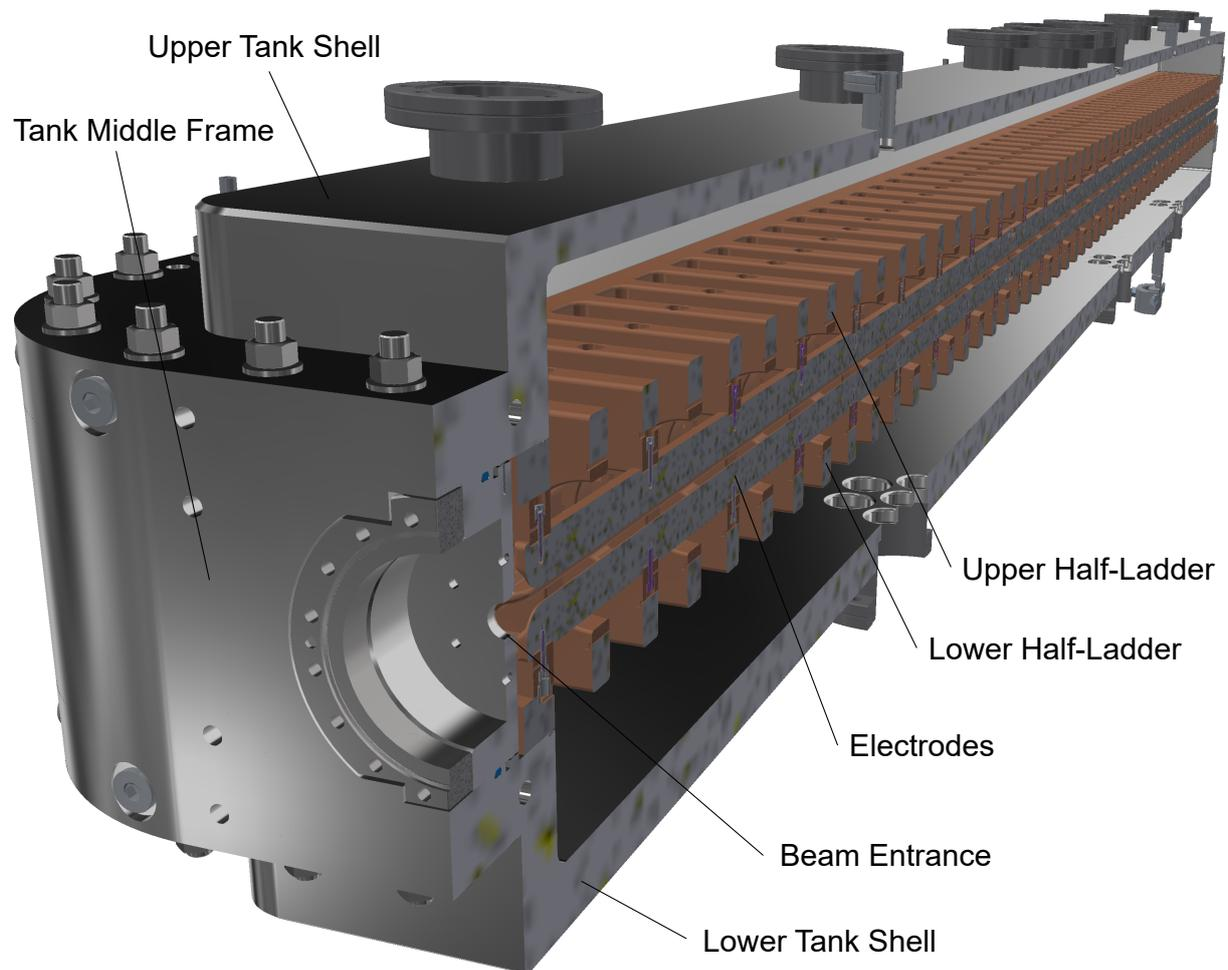
**Figure 1.** Isometric view of the 3.3m modulated Ladder-RFQ. Solid copper carrier-rings guarantee the electrode positioning as well as the RF contact. The ladder structure consists of bulk copper components. Any brazing or welding processes were avoided for the assembly of the main components.
