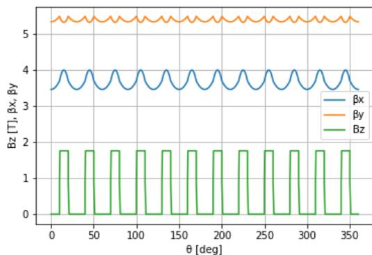
**Figure 3.** Beta functions and  $B_z$  of PPR.
