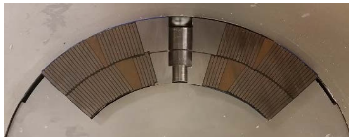
Figure 2: Cross-section and picture of a manufactured coil.
