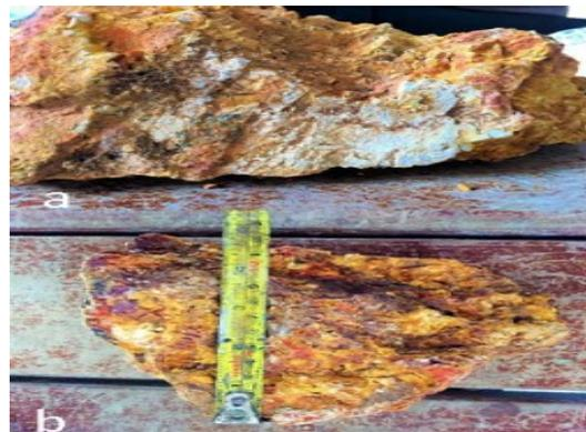
**Figure 2.** (a) Root wedges inside a rock (b) Red and violet as a sign of oxidation process occurred.
