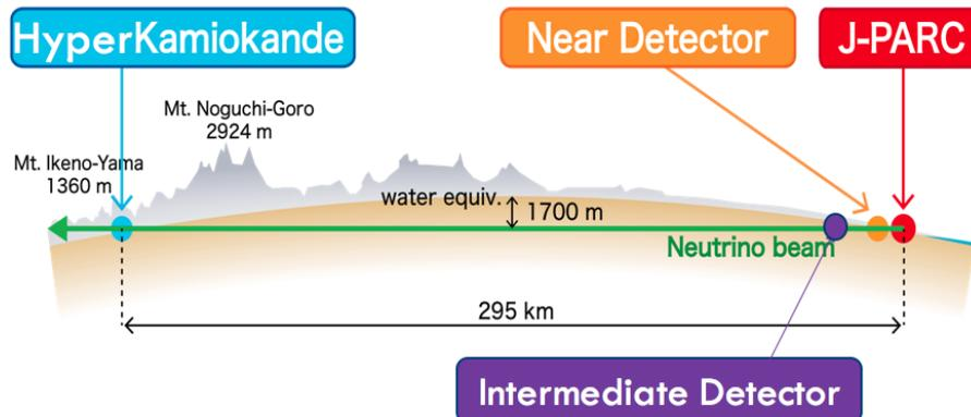
**Figure 1.** Schematic of the Hyper-K long baseline setup with far, intermediate and near detector components (not to scale).
