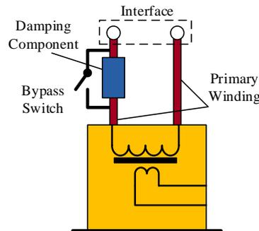
**Figure 7.** Schematic diagram of a PT with a damping component.
