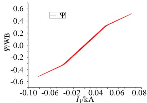
**Figure 6.** B-H curve of the potential transformer.
