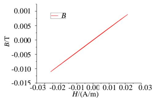
**Figure 4.** B-H curve of the current transformer.
