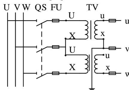
**Figure 1.** Schematic of V/V connection of potential transformers.
