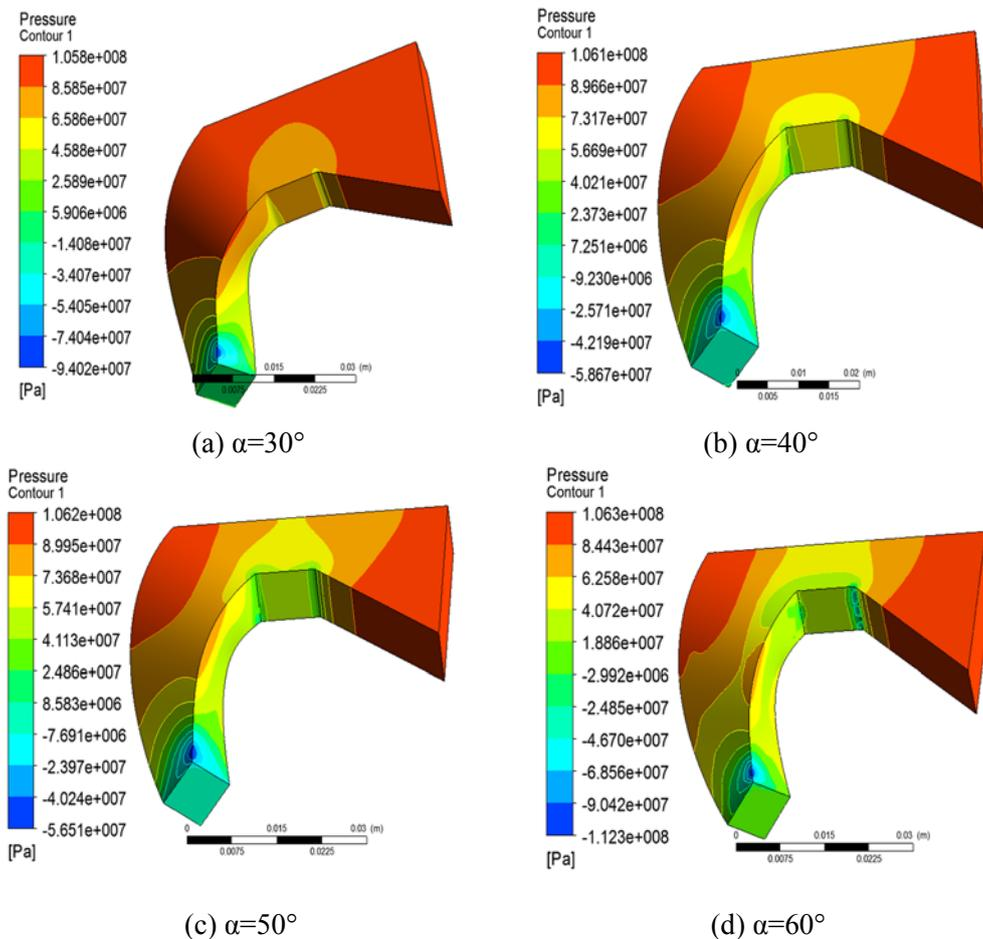
**Figure 8.** Pressure cloud diagram
