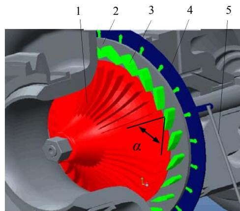
1- Turbine, 2- fixed plate, 3- guide vane, 4- control disc, 5- control rod
