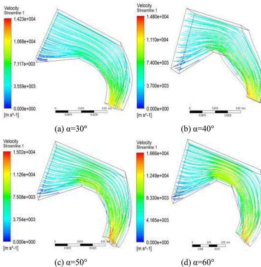
**Figure 7.** Gas velocity diagram
