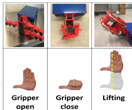
Figure 3. Hand gesture for mobile robot operation
