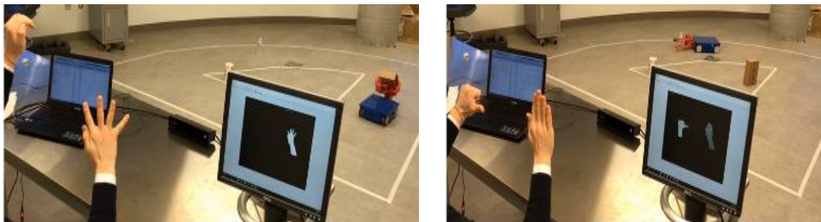
(a) To rotate the robot CCW and to lift the gripper (b) To stop the robot and to close the gripper
