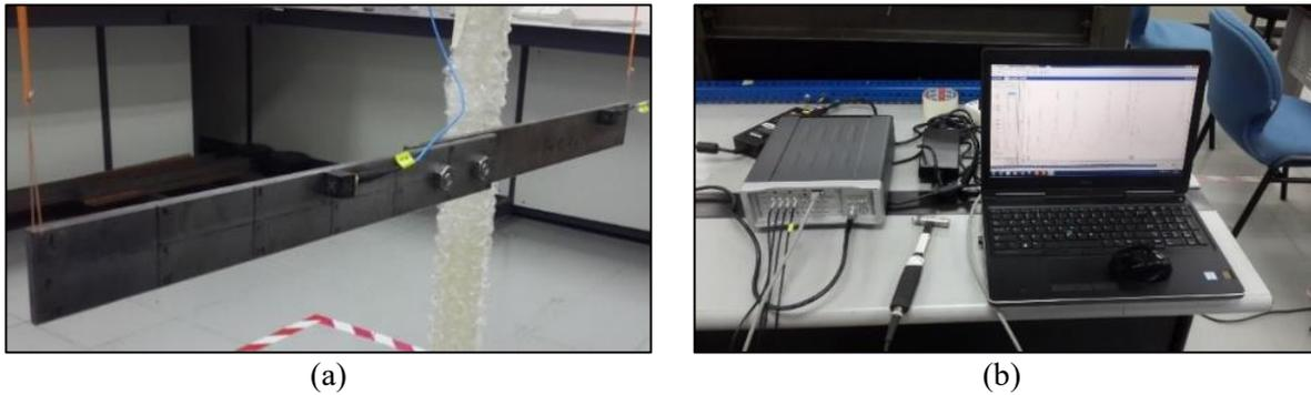
**Figure 2.** (a) Experimental set up for the assembled structure with bolted joints; (b) Testing equipment for EMA.
