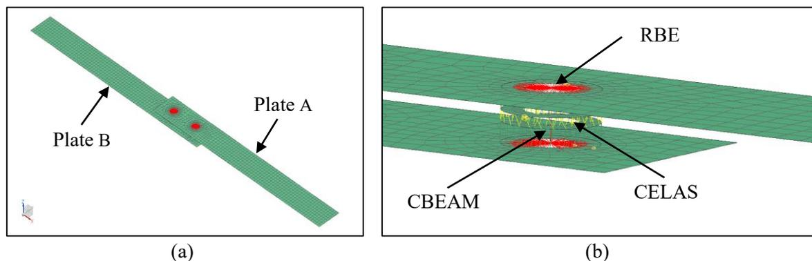
**Figure 1.** (a) Finite element model of the assembled Plate A and Plate B; (b) Representation of bolt, nut and assembly interface.
