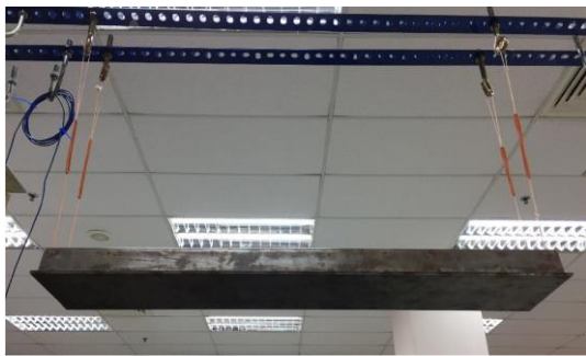
Figure 2. The structure is suspended using rubber bands and strings
