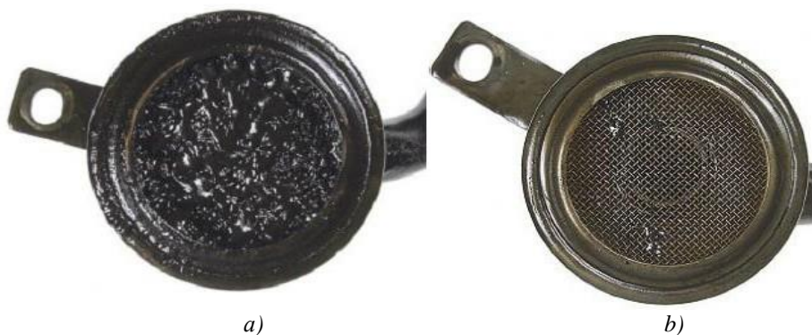
Figure 2. Typical sediments on the grid of the oil receiver: a – the grid of the oil receiver with sediments; b – the grid of the oil receiver without sediments.
