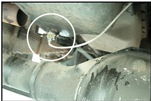
Figure 4. A drain plug with a thermocouple.
