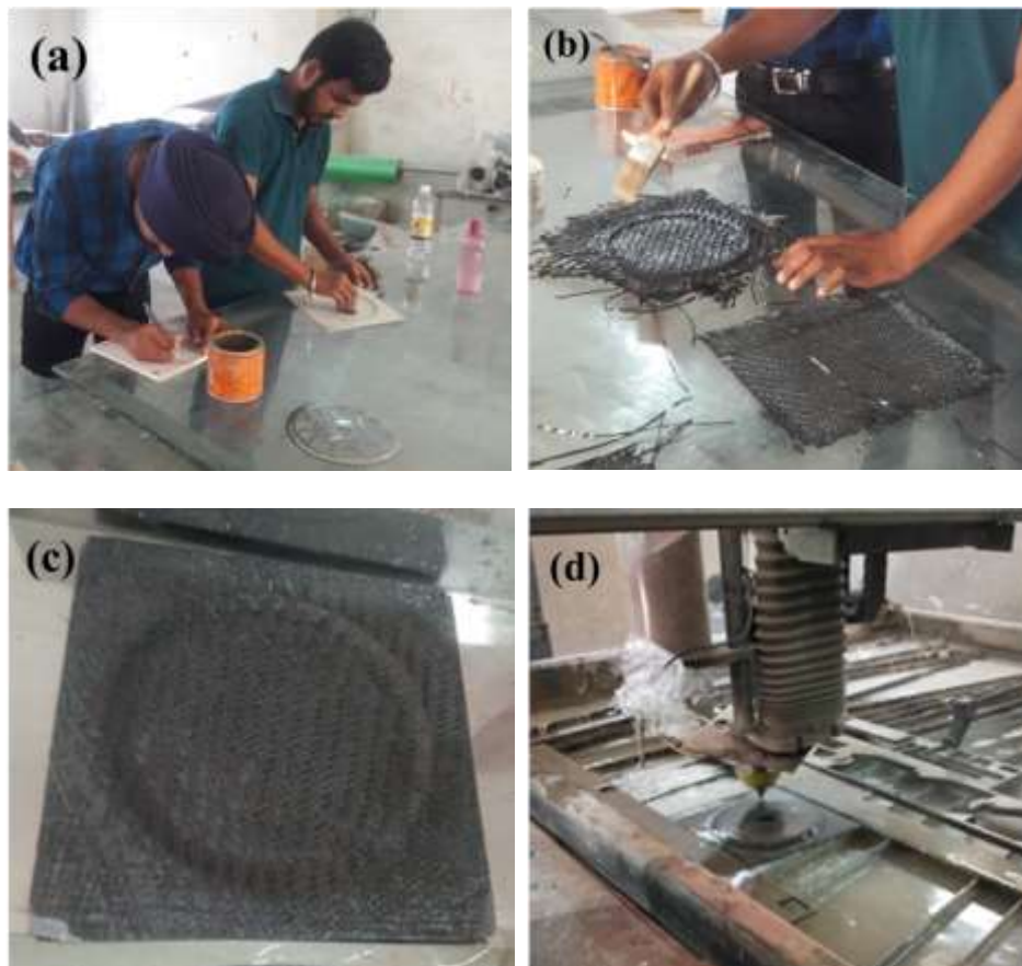
Figure 3. Sprocket manufacturing procedure (a) mould fabrication for sprocket (b) hand layup method of CFRP composite (c) finished composite (d) water jet machining for spline and teeth fabrication
