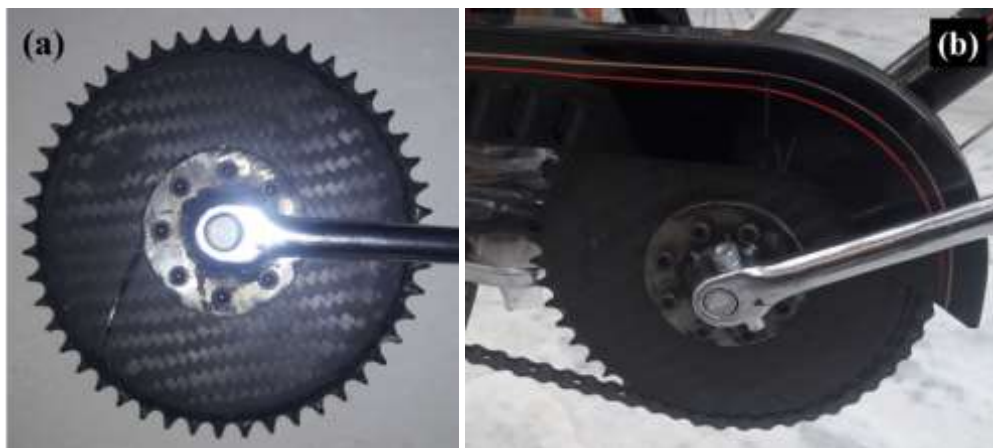
Figure 11. (a) Modified CFRP sprocket (b) fitted in cycle
