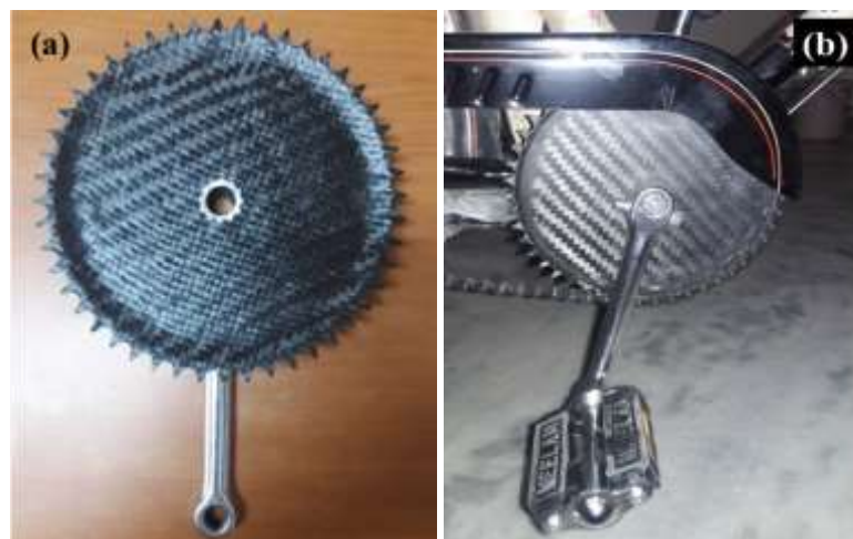
Figure 8. (a) CFRP sprocket attached with pedal shaft (b) CFRP sprocket fitted cycle
