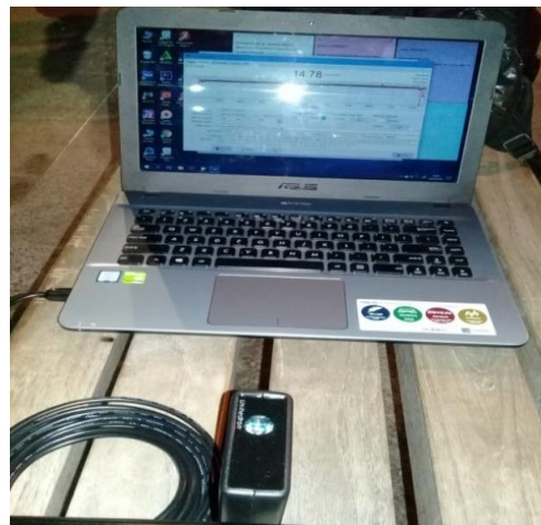
Figure 2. The design of data collection. The Sky Quality Meter (SQM) was directed to the zenith http://unihedron.com .
