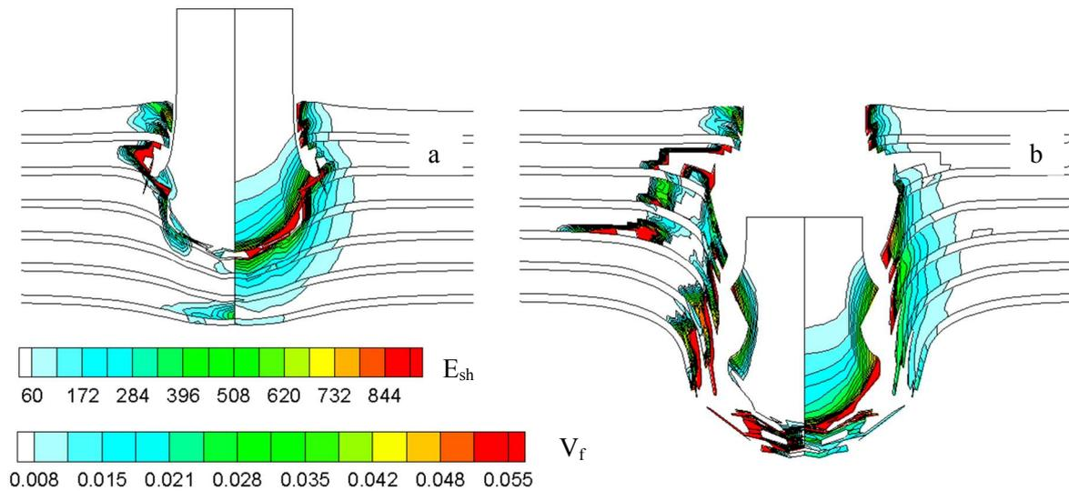
**Figure 1.** Fields of specific volume of microdamages ( $\text{cm}^3/\text{g}$ ) (left) and specific energy of shear deformations ( $\text{kJ}/\text{kg}$ ) (right) at an initial impact velocity of 2000 m/s: (a) at the time of 5.5  $\mu\text{s}$ ; (b) at the time of 10.5  $\mu\text{s}$ .
