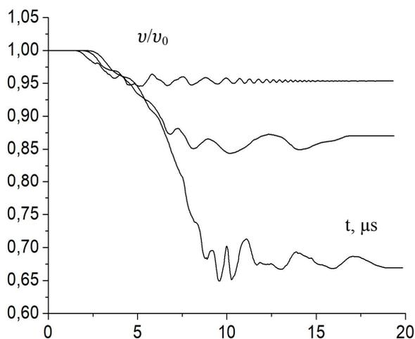
**Figure 3.** Dimensionless quantity  $v/v_0$  describing the ratio of the velocity of the rear part of the projectile to its initial velocity versus the interaction time for different initial impact velocities: (1) 2000 m/s, (2) 3000 m/s, (3) 5000 m/s.
