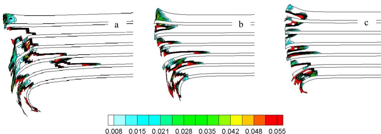
**Figure 2.** Fields of specific volume of microdamages ( $\text{cm}^3/\text{g}$ ) in targets interacting with projectiles at different initial velocities: (a) 2000 m/s; (b) 3000 m/s; (c) 5000 m/s;  $t = 20 \mu\text{s}$ .
