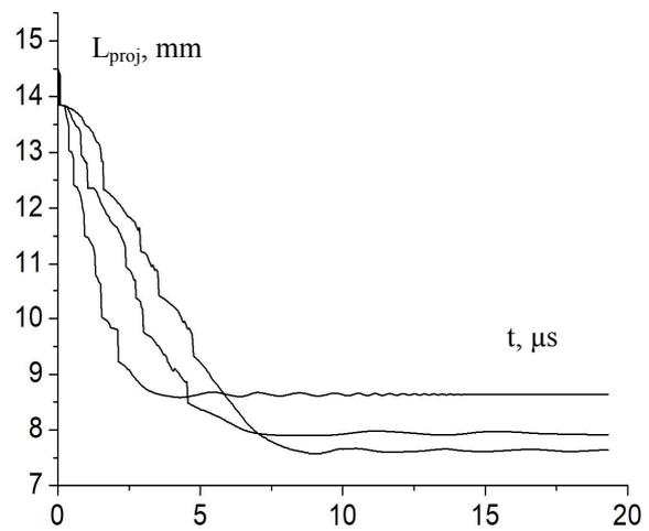
**Figure 4.** Length of the projectile as a function of time for different initial impact velocities: (1) 2000 m/s, (2) 3000 m/s, (3) 5000 m/s.
