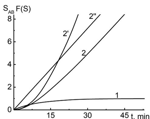
**Figure 1.** Change of the external (1) and reaction (2) specific surfaces of the mechanocomposite particle during grinding. Lines 2' and 2'' are an analytical calculation of the reaction surface  $F(S)$  using formulas (15) and (16), respectively.
