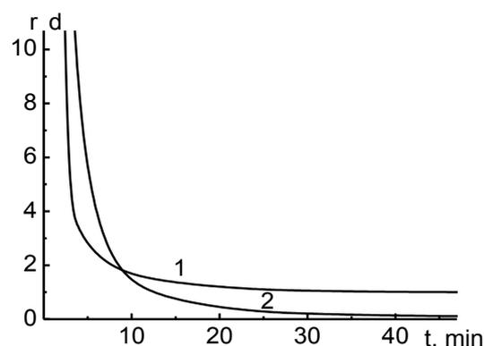
**Figure 2.** Particle size (1) and thickness of the layers of the mechanocomposite (2) during the grinding of a binary mixture.
