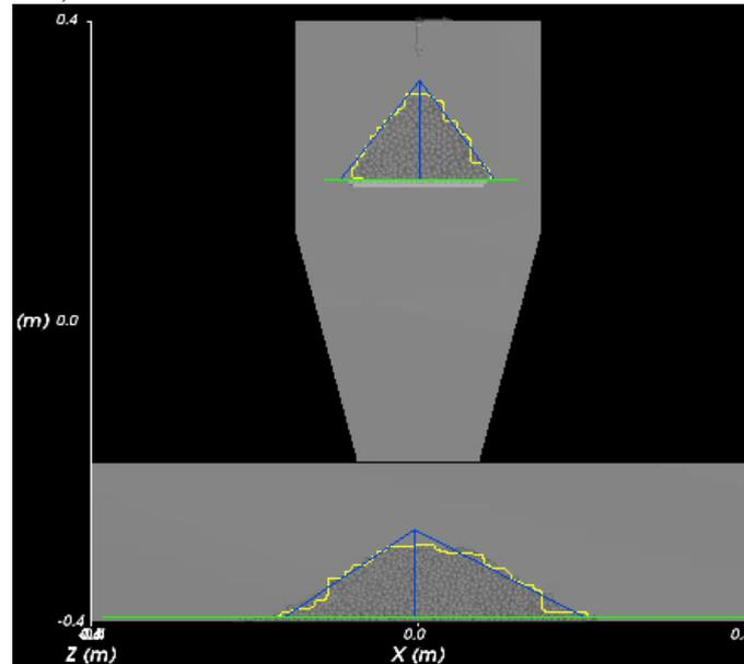
**Figure 4.** Angles of rupture and repose interpretation
