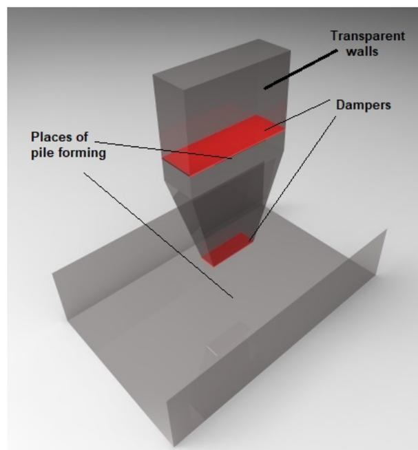
**Figure 2. Designed rig**
