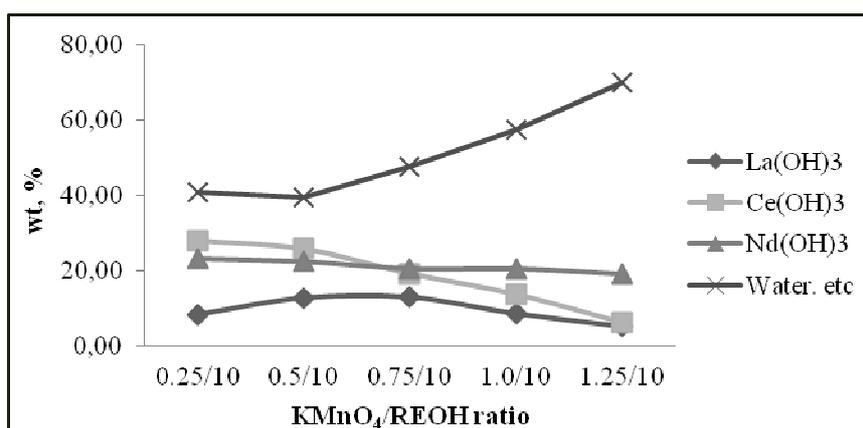
**Figure 3.** Influence of the  $\text{KMnO}_4/\text{REOH}$  ratio on the purity of the  $\text{Nd}(\text{OH})_3$  concentrate
