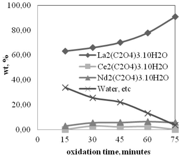
**Figure 17.** Influence of the oxidation time on the purity of the  $\text{La}_2(\text{C}_2\text{O}_4)_3$
