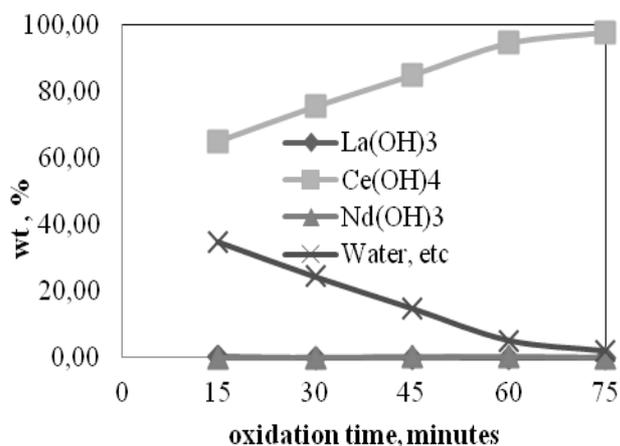
**Figure 13.** Influence of the oxidation time on the purity of the cerium hydroxide
