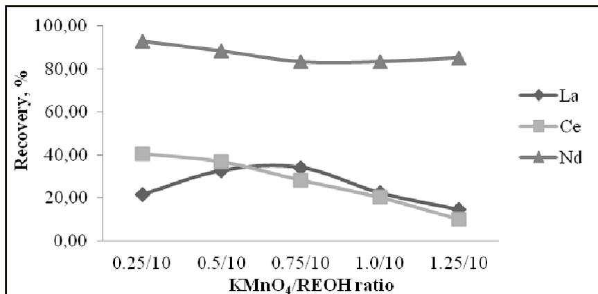
**Figure 4.** Influence of the  $\text{KMnO}_4/\text{REOH}$  ratio on the recovery of  $\text{Nd}(\text{OH})_3$
