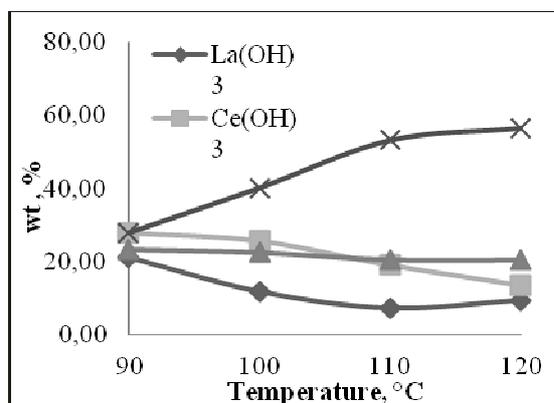
**Figure 9.** Influence of the temperature on the purity of the  $\text{Nd}(\text{OH})_3$  concentrate
