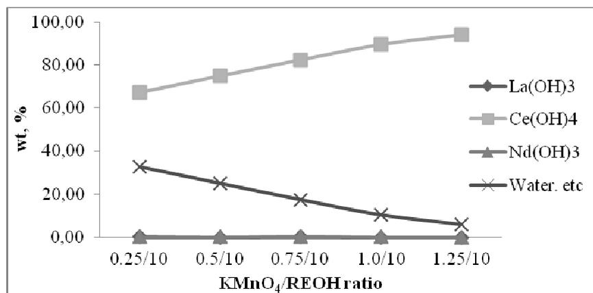
**Figure 1.** Influence of the  $\text{KMnO}_4/\text{REOH}$  ratio on the purity of the  $\text{Ce}(\text{OH})_4$
