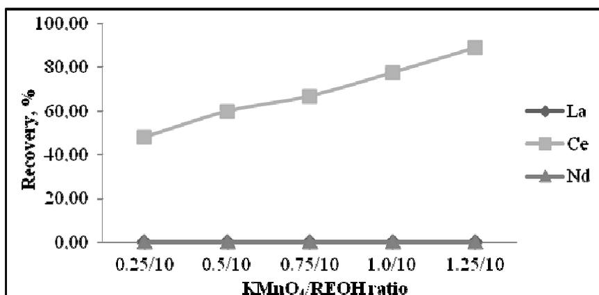
**Figure 2.** Influence of the  $\text{KMnO}_4/\text{REOH}$  ratio on the recovery of the cerium in  $\text{Ce}(\text{OH})_4$
