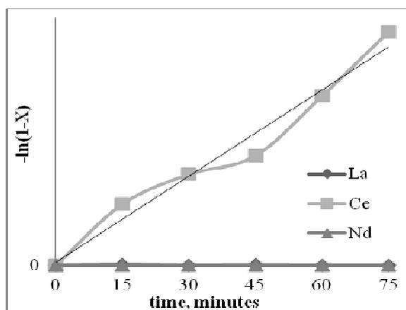
**Figure 19.** Correlation between time and  $-\ln(1-X)$  for determining of  $k$  value and linearity of first order reaction
