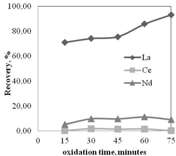
**Figure 18.** Influence of the oxidation time on the recovery of the  $\text{La}_2(\text{C}_2\text{O}_4)_3$
