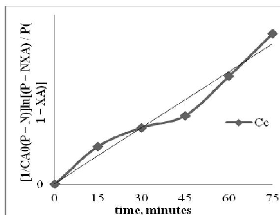
**Figure 20.** Correlation between time and  $[1/C_{A0}(P-N)] \ln[(P-NX_A)/P(1-X_A)]$  for determining  $k$  value linearity of second order
