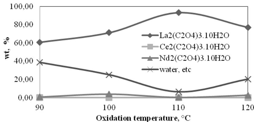
**Figure 11.** Influence of the temperature on the purity of the  $\text{La}_2(\text{C}_2\text{O}_4)_3$
