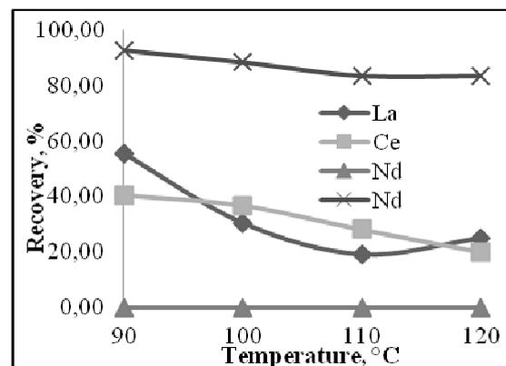
**Figure 10.** Influence of the temperature on the recovery of  $\text{Nd}(\text{OH})_3$  concentrate
