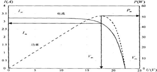
**Fig.6** Just started P - V curve diagram
