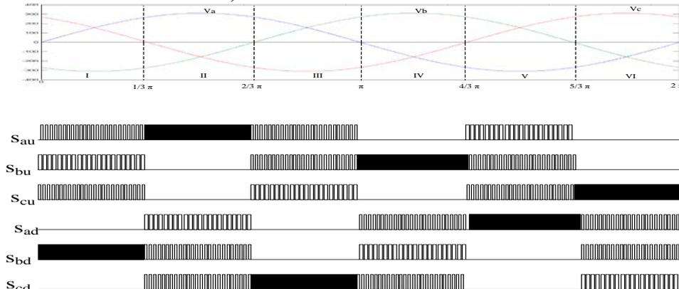
**Fig.2** Figure 6 sectors of the power supply power frequency cycle
