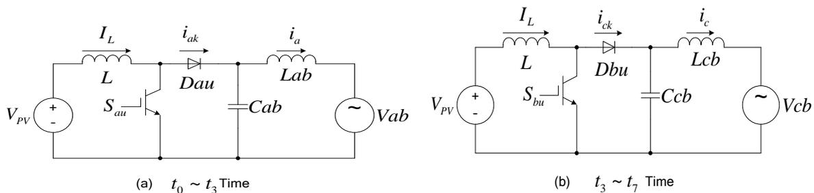
Fig.5  $t_0 \sim t_3$  and  $t_3 \sim t_7$  has two subinterval circuit model of equivalent figure
