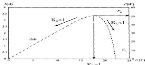
**Fig.7** P vs V plot at the stable state
