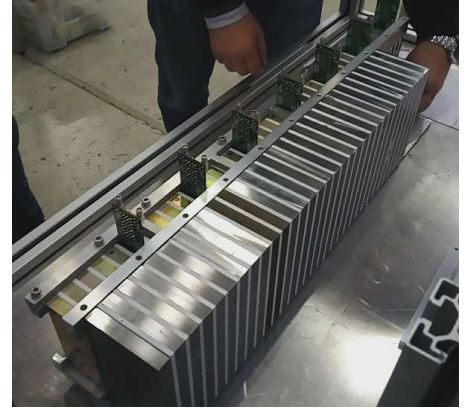
Figure 4. Photo of the calorimeter during the installation. The calorimeter is rotated by 90^\circ with respect to the layout.
