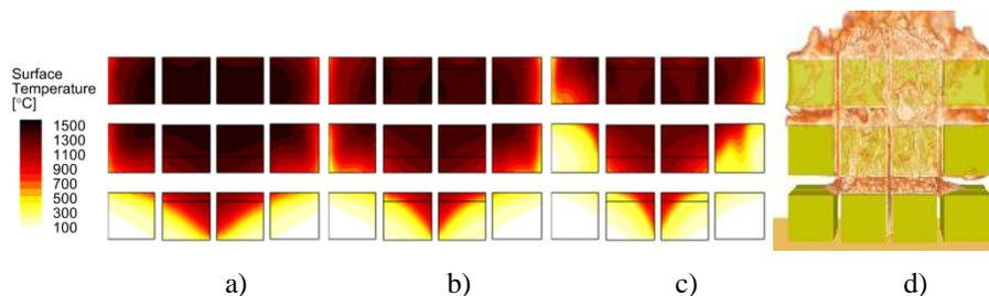
Fig. 3. The temperatures of the inner box surfaces (facing inside the rack) predicted with different values of the heat of gasification: a)  $0 \text{ MJ/kg}$ ; b)  $0.5 \text{ MJ/kg}$ ; c)  $1 \text{ MJ/kg}$  at time instant 150 s and (d) the corresponding flame snapshot ( $200 \text{ kW/m}^2$  heat release rate iso-surface, the heat of gasification-  $1 \text{ MJ/kg}$ ).
