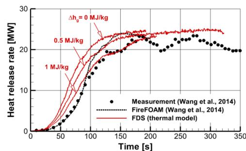
Fig. 2. Heat release rate history in the  $2 \times 4 \times 3$  rack-storage free-burn fire
