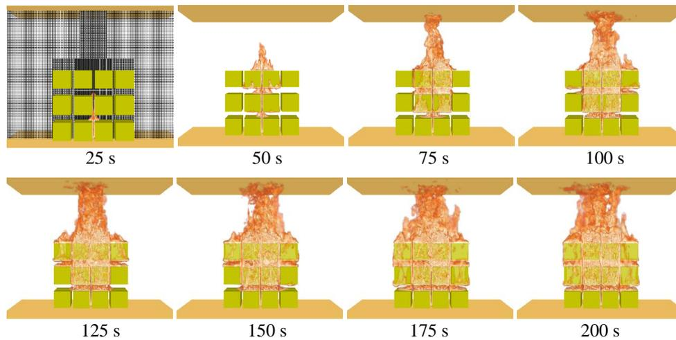
Fig. 1. Predicted flame snapshots ( $200 \text{ kW/m}^2$  heat release rate iso-surface) for the  $2 \times 4 \times 3$  rack-storage free-burn fire. The left upper figure shows the computational mesh in the central plane
