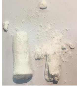
Figure 2. \beta -TCP scaffold with 10 wt. % of \beta -TCP powder
