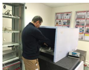
Figure 3. Setting of the relevant polygon face for optical probing of the autocollimator using the intermediate table (Moore indexing table) by manual adjustment. This is done for each n angular position setting.
