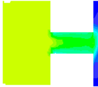
Figure 8. Measuring the total pressure of the nozzle
