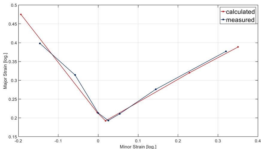
**Figure 1.** Calculated and experimental FLCs for DP600 sheet material
