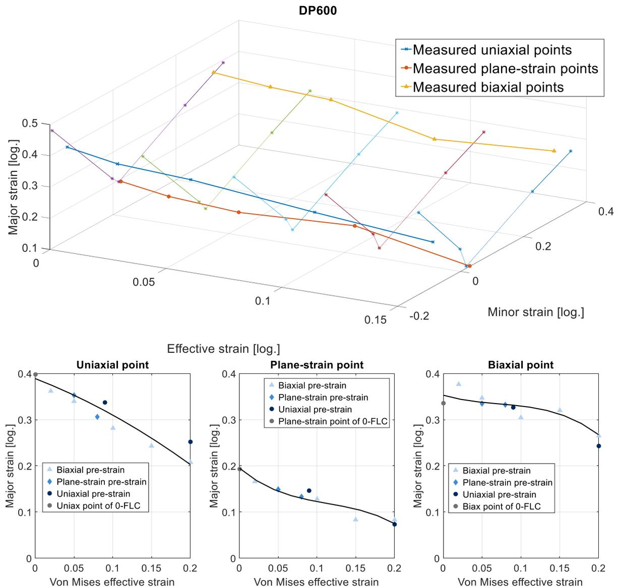
**Figure 2.** Displacement splines for uniaxial-, plane-strain and biaxial FLC point in comparison to experimental data
