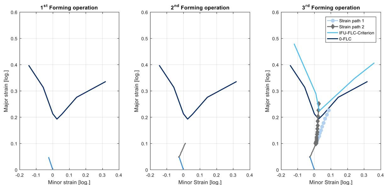
**Figure 4.** Measured evolution of strain path in forming specimen as shown in figure 3
