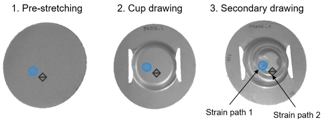
**Figure 3.** Test component formed in three drawing operations
