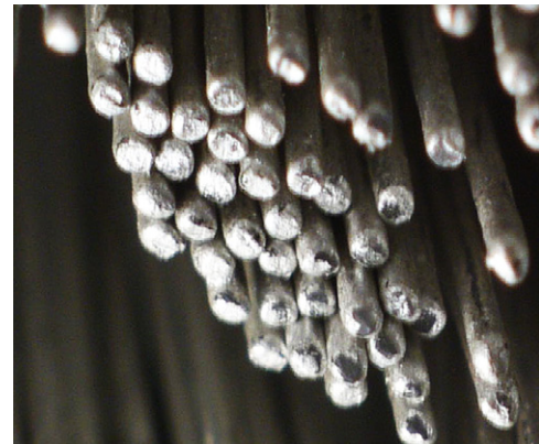
Figure 2. Macro-photograph showing the way the coating on the tips of the bristles is wearing out after months of use. The tips looking dark in this photography are no longer properly coated.
