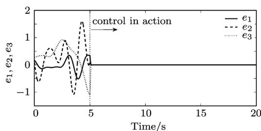
Fig. 7. State trajectories of the synchronization error system (16) with the controller of Eqs. (18) and (19).
