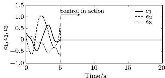
Fig. 3. State trajectories of the synchronization error system (6) with the controller of Eqs. (9) and (10).
