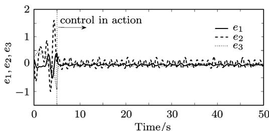
Fig. 11. State trajectories of the synchronization error system (16) with the adaptive controller in Ref. [34] and the uncertainties (20).
