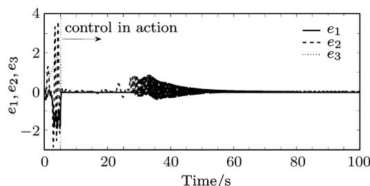
Fig. 10. State trajectories of the synchronization error system (16) with the adaptive controller in Ref. [34] and without uncertainties.
