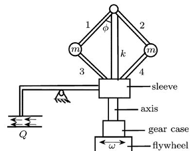
Fig. 1. Physical model of the mechanical CFG system.
