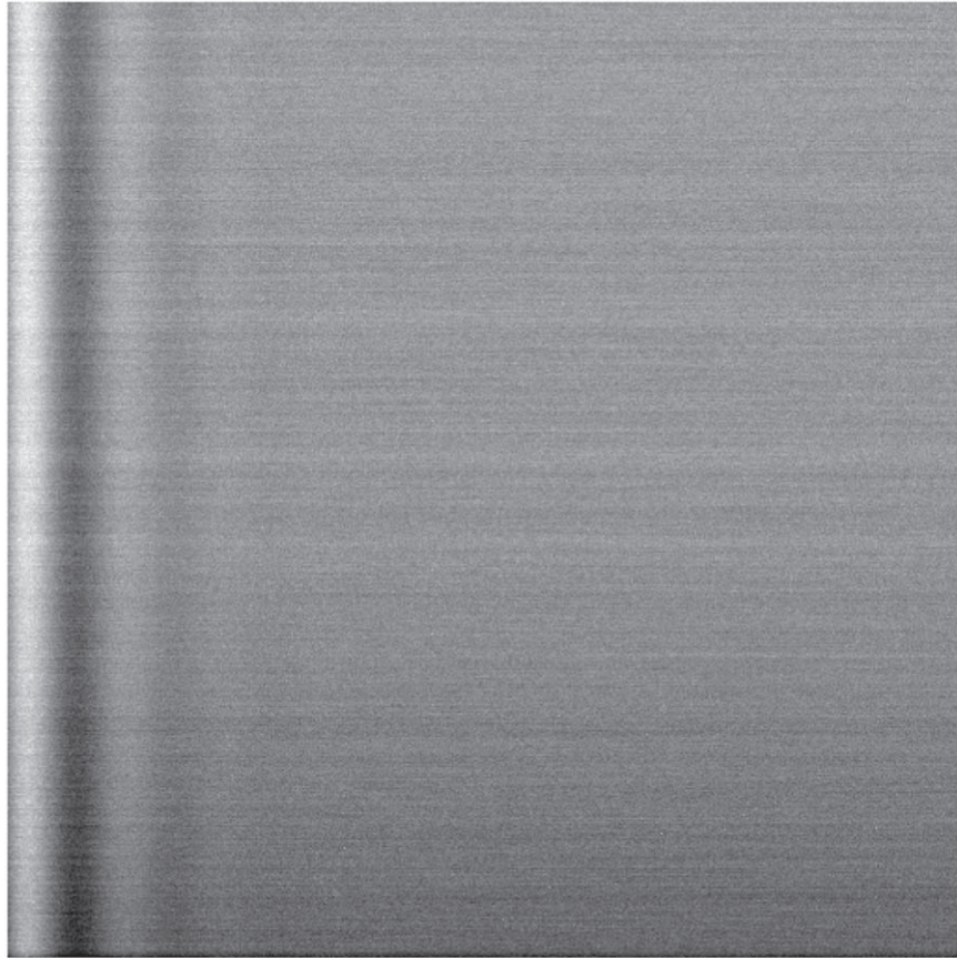
Figure 8. This “delta-bias” image, which shows the pixel-to-pixel variations in the bias level, was created by combining 100 1 \times 1 images, each with an exposure time of 0 ms, taken before the aperture door was opened. The image is displayed using a linear intensity stretch ranging from -1 to +1 DN.
