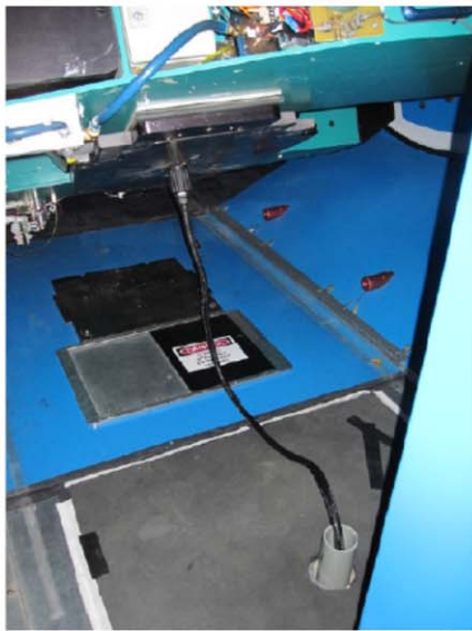
Figure 7. (Top) Gang connector “pin” during final assembly at the telescope. The ten US Conec MTP ® connectors are visible along with the interior cabling. (Middle) Model views of the gang connector “pin” and “socket.” (Bottom) The gang connector plugged into the bottom of a cartridge mounted on the telescope. The top and bottom images are from http://www.sdss.org . Images reprinted from the Sloan Digital Sky Survey under CC-BY license. (A color version of this figure is available in the online journal.)
