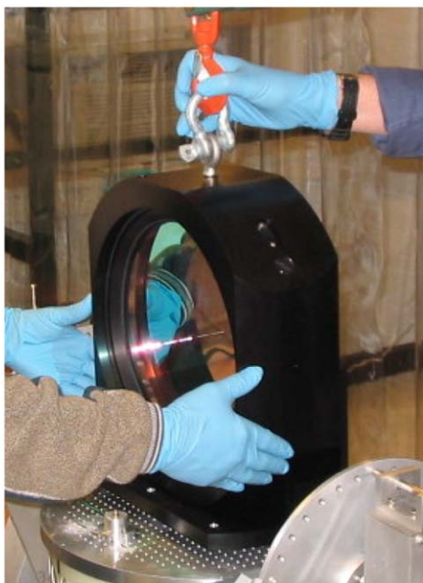
Figure 26. Camera radial support scheme was tested using a scale model of the L5 element. (Top) Reticles on the element and the cell were each monitored through cryostat windows using theodolites during a cryogenic cycle. (Bottom) The test cell as it was lowered onto the test cryostat cold plate. (A color version of this figure is available in the online journal.)
