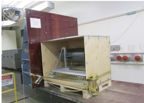
Figure 67. (Top) A model of the camera secured to the vibration isolation system of its dedicated shipping crate. (Bottom) A dummy mass model of the camera inside the shipping crate during shock and vibration testing. (A color version of this figure is available in the online journal.)
