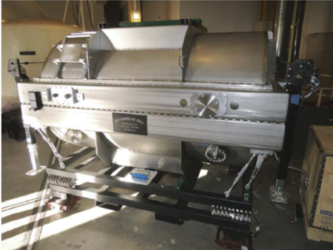
Figure 66. Custom steel shipping pallet weldment fabricated for the APOGEE-South Instrument. Wire spring isolators provide shock and vibration isolation between the lower and upper pallets. In addition to bolts which attach the lower lid of the instrument to the upper pallet, eight turnbuckles help secure the instrument and resist shear forces. The fiber spool crate is on the right. (A color version of this figure is available in the online journal.)
