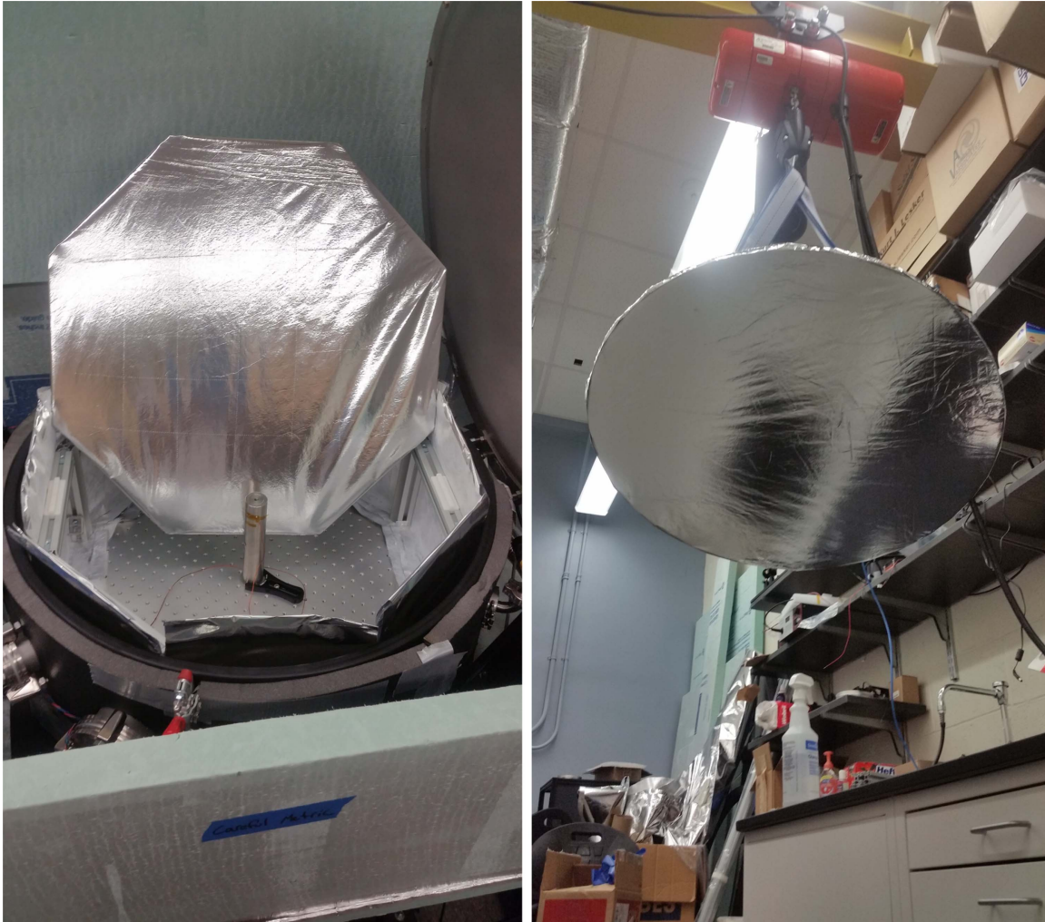
Figure 6. MINERVA-Red MLI tent being installed inside the vacuum chamber. The layers of mylar in the MLI material provide an effective barrier to radiative coupling between the vacuum chamber walls and the optical board inside the chamber.
